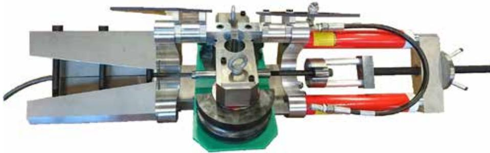
Image shows the Petersen P400 Swaging System, allowing proof load testing to be completed at time of swaging.
